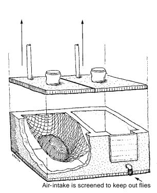
The hanging net should be pouched, not pulled tight. The net serves to expose all sides of the material to air.
