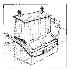
The composting toilet system can be dug into the ground. However, this should be done only where flood waters and groundwater are unlikely to flood the composter. Also, in warm climates, this makes the composter cooler than out-door temperatures, which slows the processing and creates an inviting place for insects and rodents.
