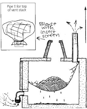
Air comes in through the air intake and out through the exhaust chimney, which should be kept as warm as possible (painted black and exposed to the sun) to promote chimney effect.
